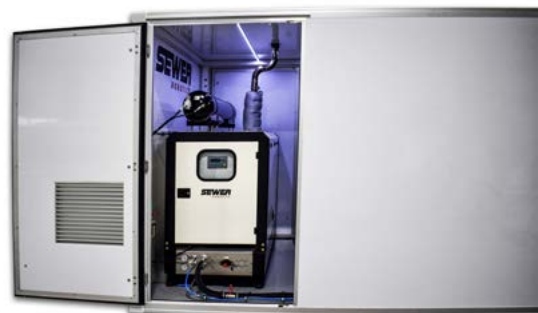
BOX INSTALLED ROBOT SYSTEM FOR 1500BAR ROBOT WATER JET CUTTING.
